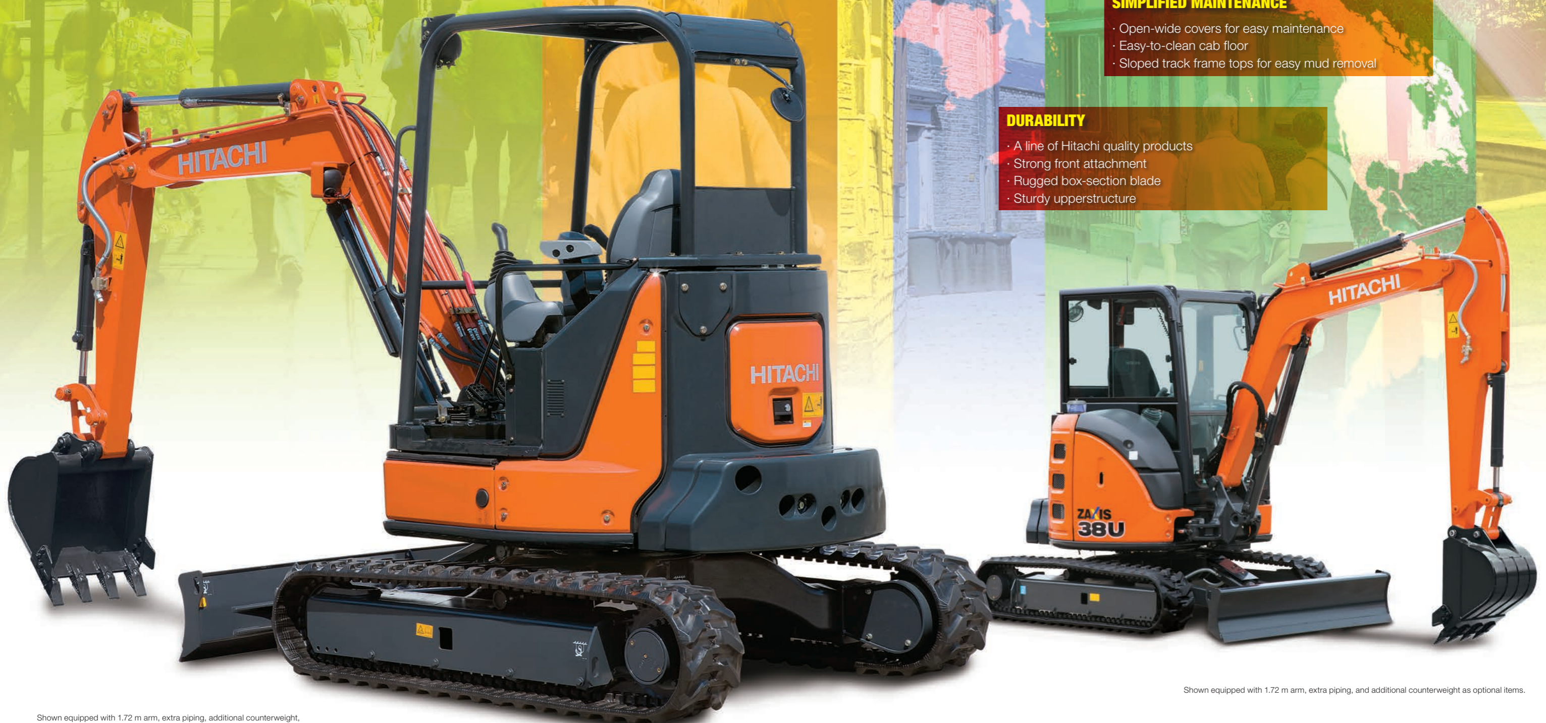
Shown equipped with 1.72 m arm, extra piping, additional counterweight, pre-cleaner and armrests as optional items.
